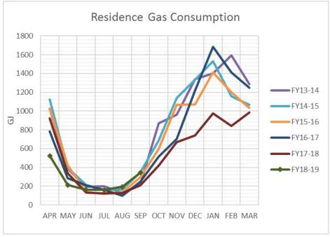
Note: Gas consumption values shown are for gas consumed within the building. Indirect gas consumption via MDES & LDES is not included in the gas plots.
