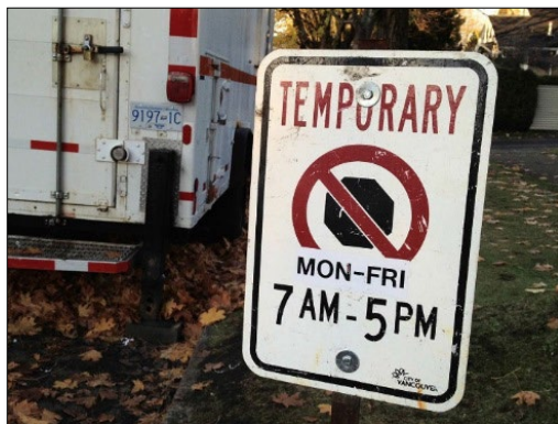
Temporary "no stopping" signs, with and without dates and times. 300 x 450 mm.
