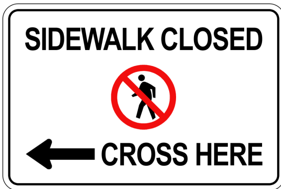
“Sidewalk closed, cross here” sign to be used at closure, or in advance of closure at intersection or location appropriate for pedestrians to cross road. 900 x 600 mm.
