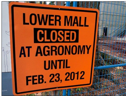
Example road closure advisory signs, with dates and times as appropriate. 900 x 600 mm or other sizes as appropriate.
