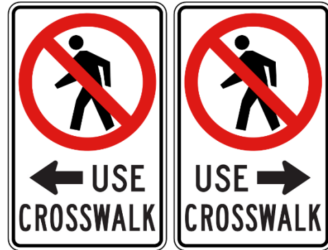
"Use crosswalk" signs to be used to direct pedestrians to crossing. 300 x 450 mm and 600 x 750 mm.
