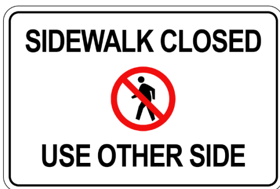
“Sidewalk closed, used other side” to be used at closure, or in advance of closure at intersection or location appropriate for pedestrians to cross road. 900 x 600 mm.
