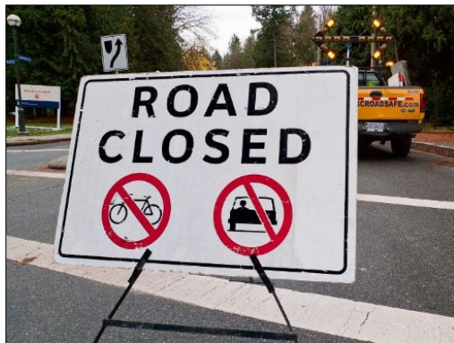
"Road closed ahead" sign to be used at intersection or decision point in advance of closure where motorists can detour around closure. 900 x 600 mm.
